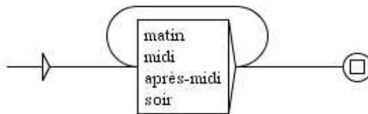
Figure 5.6: Box connected to itself
